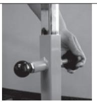
Adjust rail height by first loosening Clamping Pin by turning it 1/4 clockwise.
