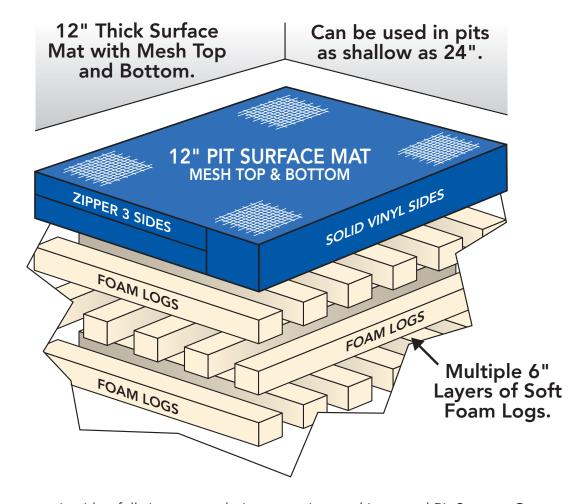
Instead of filling your pit with a full size encased pit, try our Layered Inground Pit System. Our system features base layers of soft foam logs that channel and regulate airflow. The floor level layer is a self-contained 12" mat, also filled with soft polyfoam and covered with breather mesh fabric on top and bottom. Minimum pit depth is 24", deeper pits designed to your specification.
