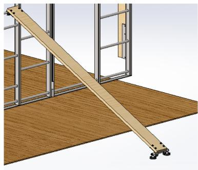
The monkey bars can fit on any rungs that are level with each other. Make sure that locks are secure. There is also a leg package for this that can be used like the plank.
