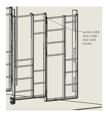
Next locate the braces. Using the bolt and nut attach the braces to the left side of the section and using the pin on the other end to attach to the right side. Some adjustment to the brace may be necessary to make sure the walls are straight. Loosen the two bolts on the end of the brace and just then tighten the bolts. With walls straight lock the wheels into place.
