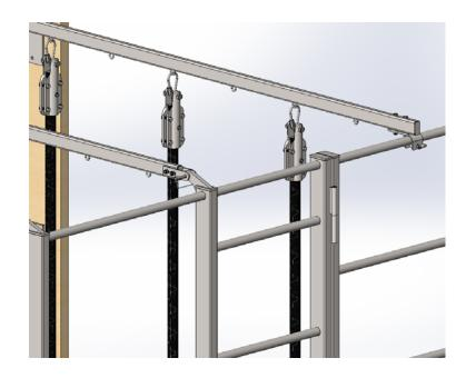
To use the rings, attach the single bar to any rungs that are at the same level with each other. To attach the bar, pull the spring lock to release the locking bar. Place over the rung and swing the locking bar up and pull the spring lock and align the locking plate hole up with the spring lock and let it snap into place. Hang the rings using the pear shaped quick link and tighten.
